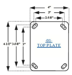
Our most popular medium duty to heavy duty semi-pneumatic caster right now is our solid polyurethane foam wheel with precision ball bearings swivel and rigid casters. These casters have case hardened double ball raceways providing extra capacity and durability. Silver Zinc plated finish. Top plate and legs are ¼" thick steel. These casters are best for manual push / pull applications.... Not motorized towing unless at very low speeds.
